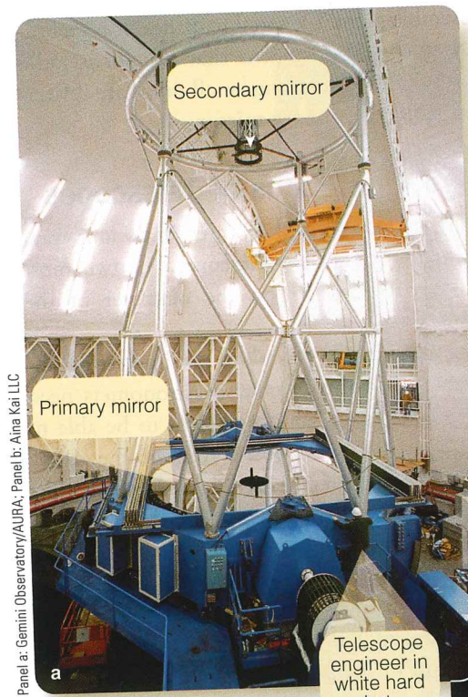
◀ Figure 6-8 (a) The Gemini-North optical telescope on Mauna Kea in Hawai'i stands more than 19 m (62 ft) high when pointed straight up. The primary mirror (at bottom) is 8.1 m (26.5 ft) in diameter—larger than some classrooms. The sides of the telescope dome can be opened, allowing quick equalization of inside and outside temperatures at sunset, reducing air turbulence and improving seeing. (b) The largest fully steerable radio telescope in the world is at the National Radio Astronomy Observatory in Green Bank, West Virginia. The telescope stands higher than the Statue of Liberty and has a reflecting surface 100 \times 110 m ( 330 \times 360 ft) in diameter, more than big enough to hold an entire football field. Its surface consists of 2004 computer-controlled panels that adjust to maintain the shape of the reflecting surface.
