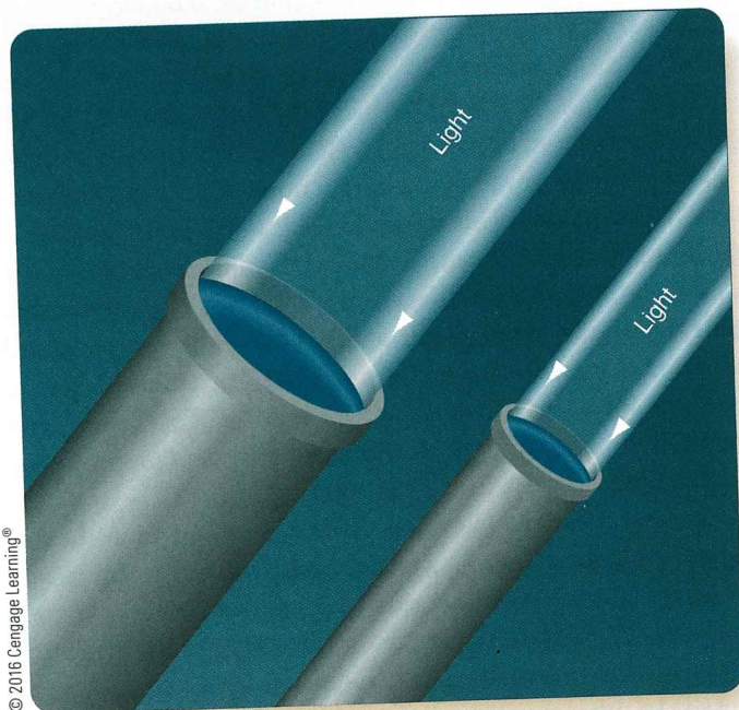
▲ Figure 6-9 Gathering light is like catching rain in a bucket. A large-diameter telescope gathers more light and produces a brighter image than a smaller telescope of the same focal length.
